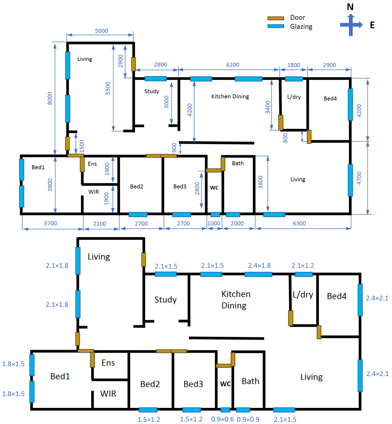
Figure 10: Floor plans of the archetypal house showing room dimensions (top), and glazing dimensions (bottom); adapted from [22].
