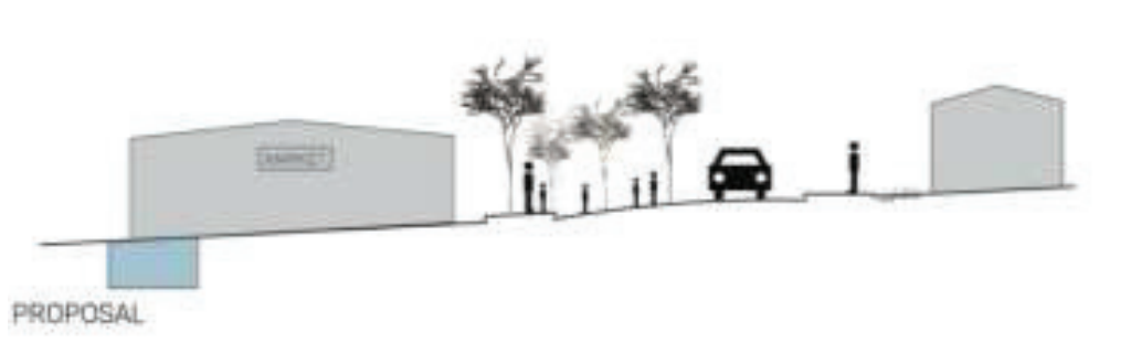
Figure 41. 4-domains approach of flood resilience (4DA), third domain shows the design of an underground water retention
