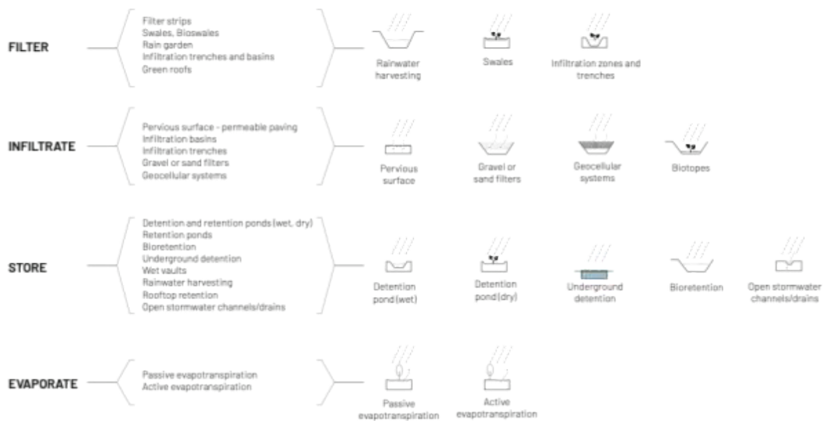
Figure 14. Low Impact Design (LID) + Sustainable Urban Drainage System (SUDs) practices: filter, infiltrate, store, evaporate
