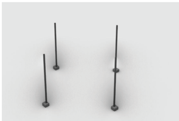
Figure 53. Bamboo columns with concrete footing
