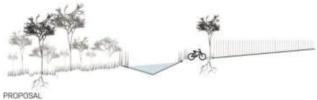
Figure 42. 4-domains approach of flood resilience (4DA), fourth domain shows the design of a floodable space in the form of a forest pocket
